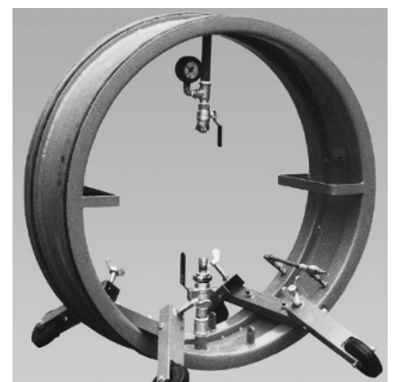
Photo: Pneumatic jointing test machine
